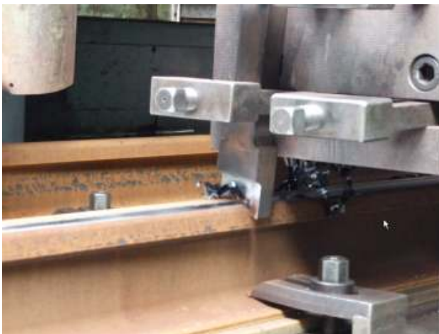
Figure 7, machining the anti-squeal rail profile.
