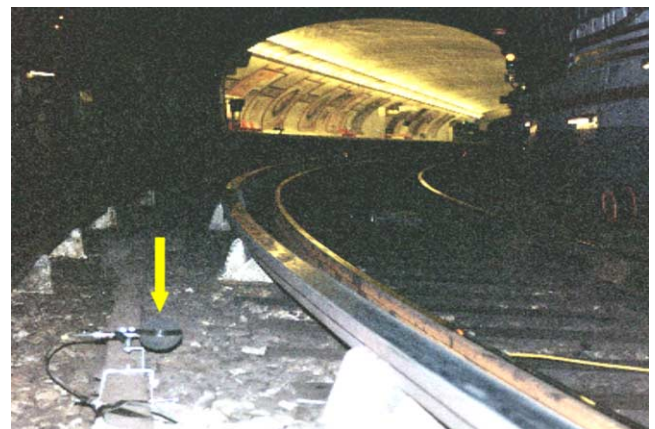
Fig. 6. Measuring position at test site (arrow points out microphone).
