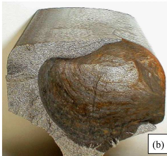
Fig. 2. (a) Head check cracking at gauge corner (top view of railhead); (b) transverse rail fracture from a head check.
